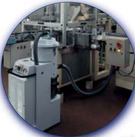
Spot suction on a production line.
