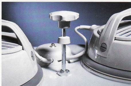
Filter shaker to regenerate the large filter, ensuring a constant airflow.
