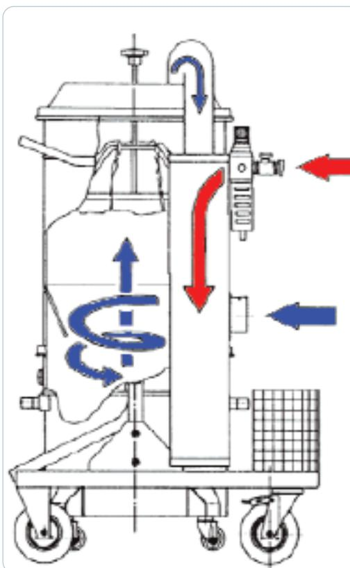
The compressed air passes through the pressure gauge and compressed air filter and is then channelled downwards into the "Venturi tube". By quickly passing through it, it creates a vacuum inside the entire unit, through the pipe in the head. In this way we suck air through the inlet (blue arrow), which then goes into the filter chamber, through the filter and down the "Venturi tube" where it joins the compressed air (red arrow).
