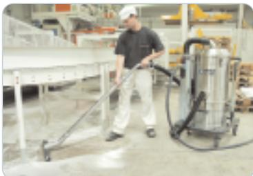
Compressed air vacuums are the ideal solution in ATEX zoned areas, for maintenance, general cleaning, and for collection of organic and metallic dusts, and swarf containing explosive vapours.
